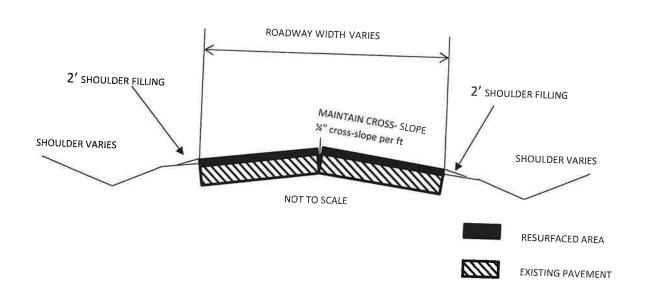
RETAIN EXISTING PAVEMENT AND MAINTAIN PROPER CROSS SLOPE. PATCHING AND LEVEL 85 LBS PER SQUARE YARD OR AS DIRECTED BY ENGINEER. RESURFACE FULL WIDTH WITH 135 LBS PER SQUARE YARD RECYCLED ASPHALTIC CONCRETE 9.5MM SUPERPAVE, GP 2 ONLY, INCL BITUM MATL & H LIME.
