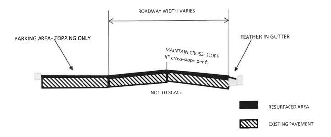
RETAIN EXISTING PAVEMENT AND MAINTAIN PROPER CROSS SLOPE. PATCHING AND LEVEL 85 LBS PER SQUARE YARD OR AS DIRECTED BY ENGINEER. RESURFACE FULL WIDTH WITH 135 LBS PER SQUARE YARD RECYCLED ASPHALTIC CONCRETE 9.5MM SUPERPAVE, GP 2 ONLY, INCL BITUM MATL & H LIME.
